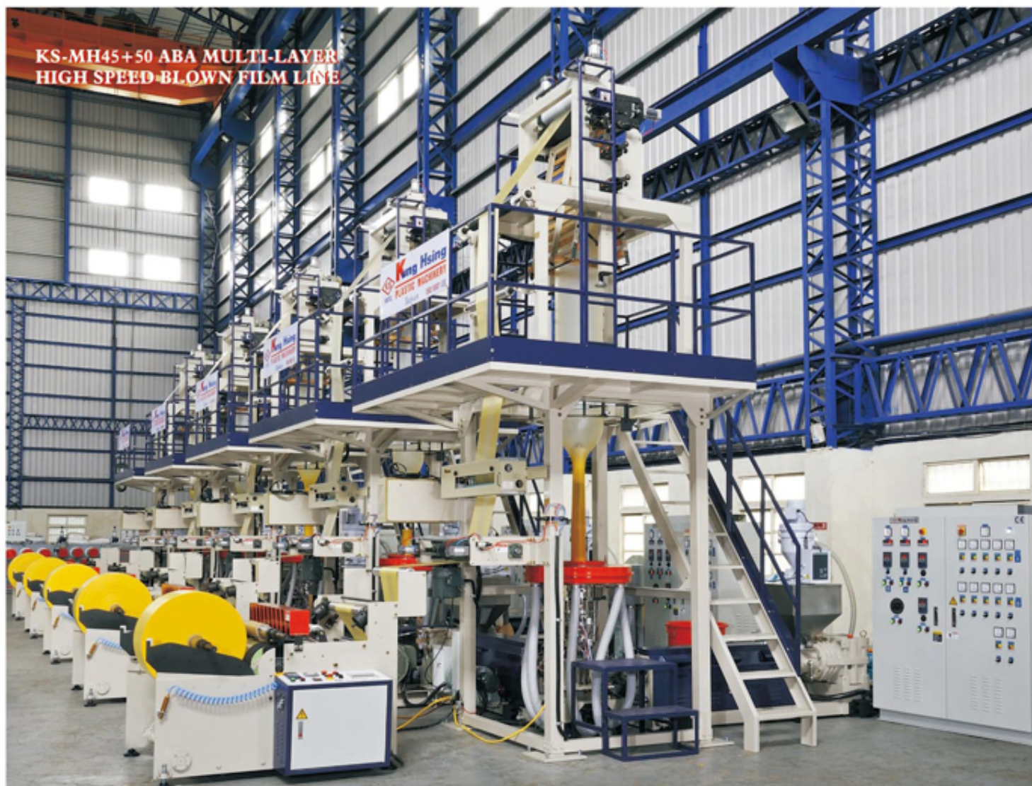
KS-MH55+65 ABA MULTI-LAYER HIGH SPEED BLOWN FILM LINE INCLUDING VERTICAL TYPE OSCILLATING TAKE UP UNIT & EPC
