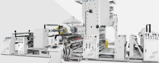
Anchor coating unit with high efficiency drying nozzles
