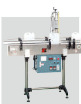
測漏機 Leaking Tester
