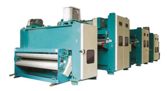
A complete needle punching section including feeding system, pre-needle punching machine, finish needle punching machine, edge cutter, and other peripheral equipment. Taylor made complete needle punching line according to customer's needs leads to great flexibility of production. Wide range of application covers geotextile, car carpet, filtration, mattress, and more.
