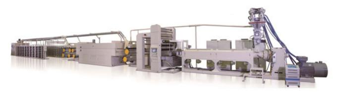
One layer extrusion tape line for PP, or HDPE flat tapes. With melting capacity from 120kg/hour to 700kg/hour, producing films width from 460mm to 1400mm. Tape Winding speed from 250m/min to 450 m/min, which produces premium quality tapes for use in woven sack, Kraft Paper cement sack, PE Tarpaulins, and various applications.
