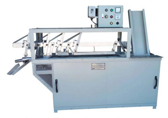
Dedicated design for removing waste yarn on bobbins with high efficiency
