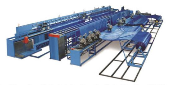
Our automatic tarpaulin making line is designed to weld multiple rolls together with 2 side eyeleting, and cut to desired length simultaneously.
