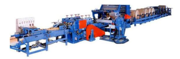
Automatic tubing process produces multi-ply printed Kraft Paper bags in 1 line. Applications of gusset and valve forming available on the same line. Inline flexographic printing from 1 to 4 color.
