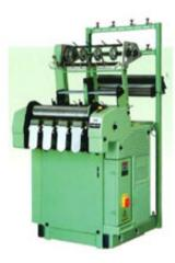
High speed automatic needle loom dedicated for producing carrying belt and filler cord used for FIBC.
