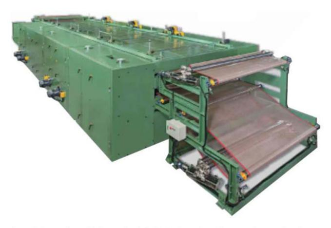
A complete pressing and drying section including heat pressing rollers, oven dryer, embossing rollers, cooling system, accumulator, cutters, winders, and other peripheral equipment. It furnishes the final product with different extent of hardness and touches.
