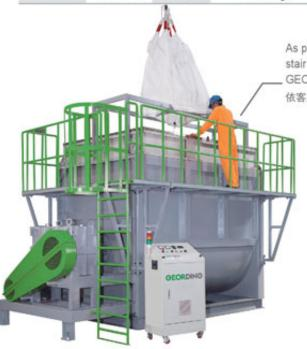
As per client's requirement, has been set a safety stair to let operator give a much easier maintenance. GEORDING helps to customize super huge tank. 依客戶要求製作安全樓梯,便於維修與保養。
