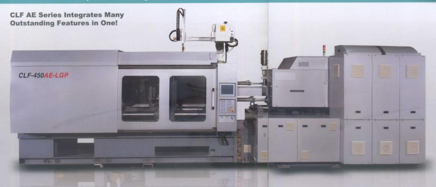
With extra low speed and extra high speed injection controls to suit molding requirements for optical products and LPG. Also suitable for thin-wall production with shortened cycle time to greatly reduce production costs.
